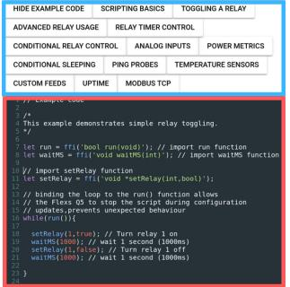
All scripting is managed as a secondary priority to the main functions of the Q5 (to avoid interruptions to system tasks). For a more in-depth look at scripting, please see the on board examples.
