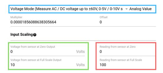
Set the sensor range using the specs found on the side of the sensor or in the provided data sheet. In the above example, 0V corresponds to 0 PSI and 10V corresponds to 100 PSI. Enter the voltage output range of the sensor's analog output in the green box. If the sensor output was a 0-5V signal level, the values in the green box would be 0 and 5 instead of 0 and 10.
