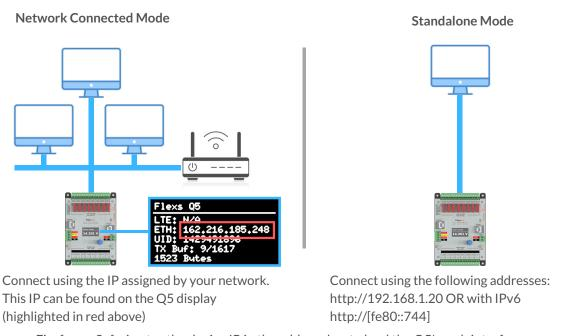
Using Chrome, Firefox or Safari enter the device IP in the address bar to load the Q5's web interface.
