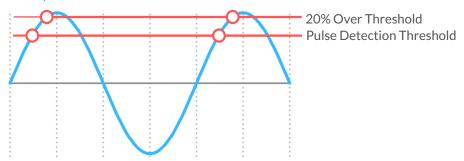
Frequency is the number of valid pulses per second or hertz (Hz).
