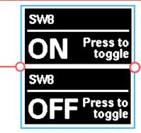
Load Relay Page - Press the knob to switch relay ON/OFF. See Section 3.0 for more info on naming relay channels.
