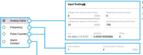
For additional information on the Analog Value option and Input Scaling calculator refer to sections 2.1 and 2.2.
