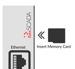
The Q5's internal memory allows for roughly 1 month\* of readings to be stored before older data is erased. In applications where extensive long term data-logging is required the Q5 may be outfitted with an external memory card for additional capacity. For more info on how to use this feature please contact FlexSCADA.
