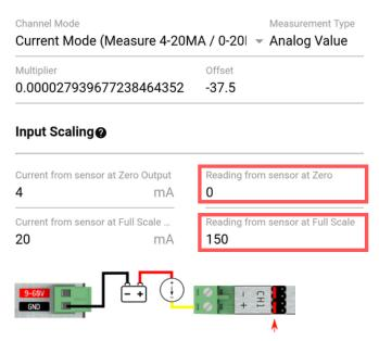
Hardware configuration example for a 4 - 20 mA sensor.
