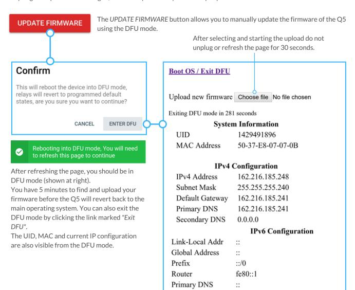
It is also possible to manually force the device into DFU mode by holding the control knob down while power is applied to the device. This is also mentioned in Section 7.0.
