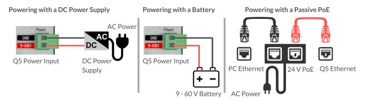
Once power is connected, the Q5 display will illuminate indicating that the Q5 has successfully started. The Q5 will then search for a router on the network to get an IP address. If the Q5 fails to find a router within the first 10s of bootup, it will fallback to standalone mode. In standalone mode, the Q5 will use the fallback IP (default 192.168.1.20).
